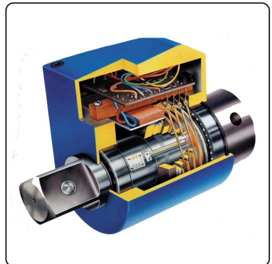
An internal view of a typical standard rotary torque transducer.
