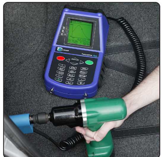
A rotary torque transducer and torque data collector being used during a quality audit test of a joint and fastener within the automotive industry.
